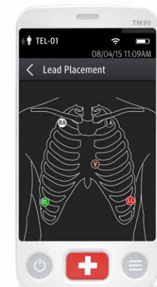
ECG lead-off guide, helps nurse locate the lead that is not properly connected.
